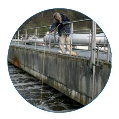
"We use our HQ30D to measure oxygen (LD0). With the 15-metre-long cable and the rugged outdoor electrode we can access all the measurement locations without difficulty. Besides occasionally checking our process probes, we use the HQD system primarily for measurements, such as the determination of LD0 at a variety of points and depths in the aeration tanks. We are especially happy with the rapid stabilisation of the reading and the fast availability of the result."
