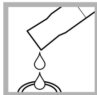
**12.** Pour 10-mL of the solution from the mixing cylinder into a second sample cell.
