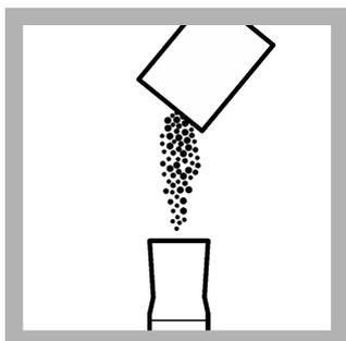
**9.** Add the contents of one Sodium Thiosulfate Reagent Powder Pillow to the remaining solution in the mixing cylinder. Make sure to prepare a blank for each sample.
