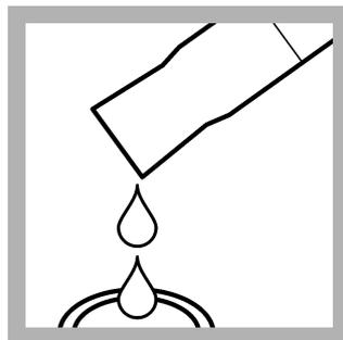
**7. Prepare the sample:** Pour 10 mL of the solution from the mixing cylinder into a sample cell.
