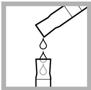
**5.** If the sample was preserved with acid, make sure that the sample pH is 9–10. Use a graduated cylinder to add 50 mL of sample to the mixing cylinder.
