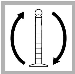
**6.** Put the stopper on the mixing cylinder. Continuously invert the mixing cylinder for 1 minute.
