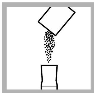
**2. Add the contents of one Silver 1 Powder Pillow to a dry 50-mL mixing cylinder.** If the powder becomes wet, it will not fully dissolve and the color will not fully develop.
