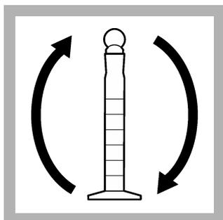
**10.** Put the stopper on the mixing cylinder. Invert the mixing cylinder several times to mix.
