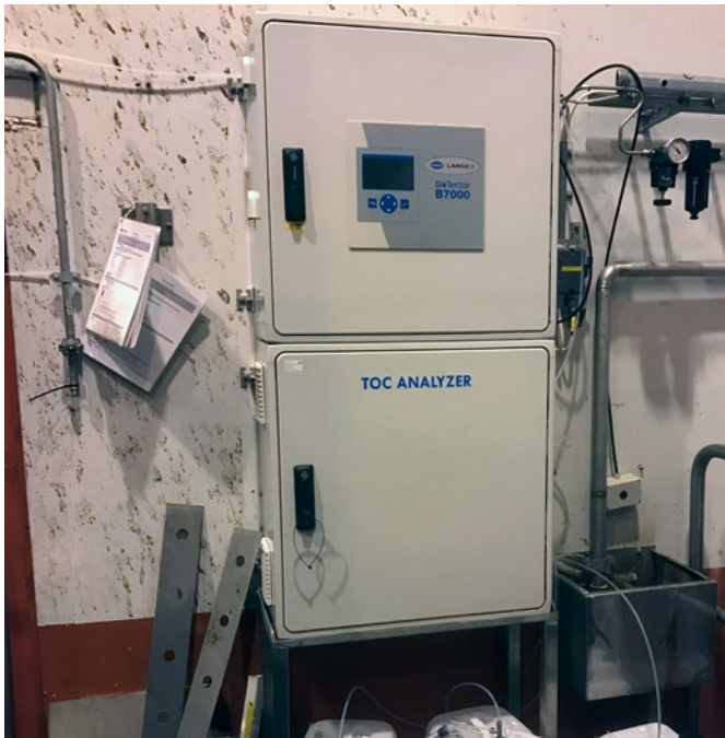
TOC analyser BioTector B7000 has a unique double oxidation method giving a total digestion of the sample, and it can handle particle sizes up to 2 mm.
