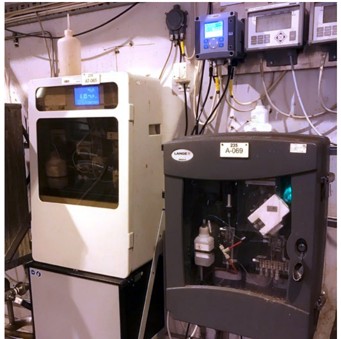
The phosphoric analyser Phosphax sigma is capable of measuring both phosphate and total phosphorus. The ammonia analyser Amtax sc is seen here with a Plexiglas door for indoor mounting.
